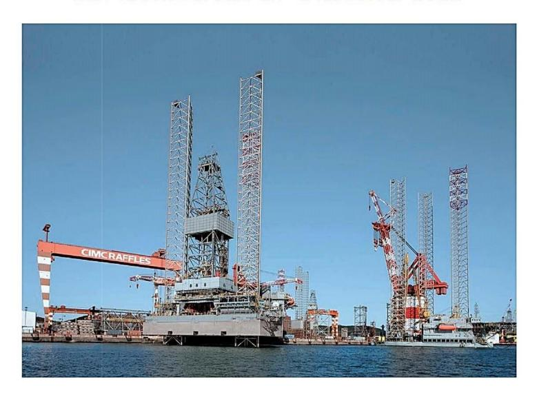
The Super M2 is a self-elevating drilling unit, designed for all year benign conditions in accordance with ABS assessment criteria. It is based on the F&G L780 Mod II jackup design.
