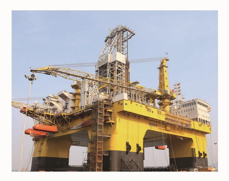
Frigstad D90 is an ultra deepwater drilling unit built by CIMC Raffles. It is able to operate in water depth of 3,658m, and drilling depth up to 15,250m. It is designed with dual hoisting tower and facilities with DP3 system and preliminary mooring
